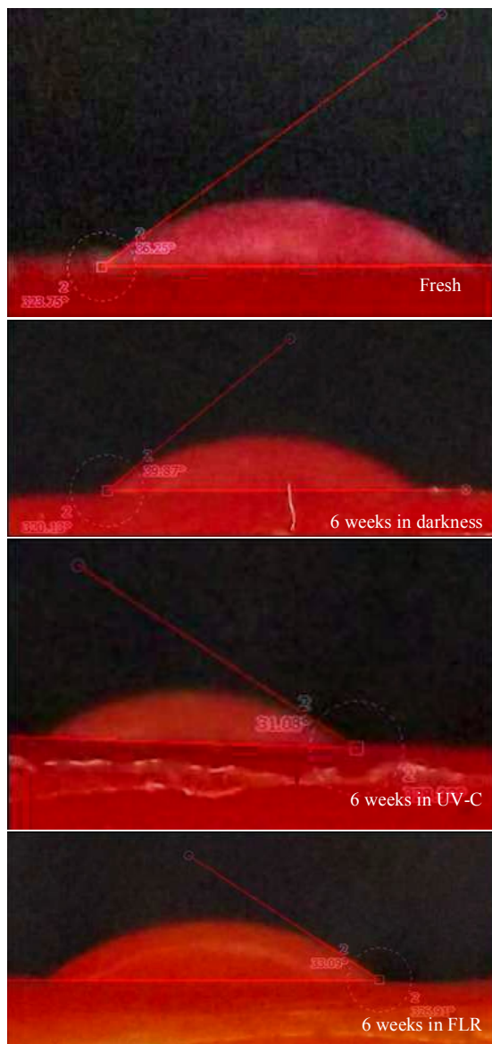
Figure 1. Contact angles of reconstituted epicuticular wax dispensed on the red pepper fruits dewaxed skin
